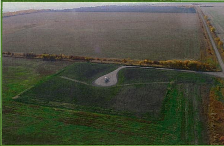
This well site has been "tear dropped", enabling farming to continue. Note access is along the field edge to minimize disruption to cultivation
